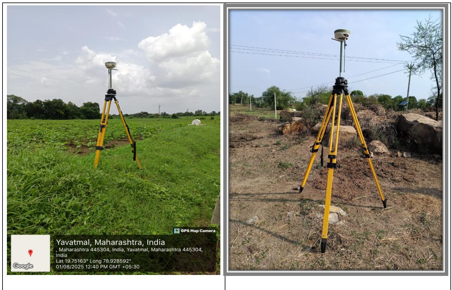
Fig.5.2: A Differential Global Positioning System (DGPS) survey at Gadeghat-Khatra block
